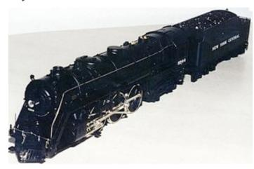
over several decades, railroads first burned wood, then lignite, soft coal, hard coal and various grades of oil to heat water to make steam. Both fuel and water were carried in a car directly behind the combustion chamber. We call that car the tender. It's always behind.
