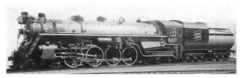
A round Vanderbuilt tender was an efficient and strong structure. This made considerable sense when oil came along as a cleaner fuel. The photo above shows the round Vanderbuilt
